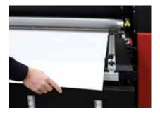
Embedded continuous print solution enhances productivity in rigid mode as it narrows down the gap between two consecutive boards
